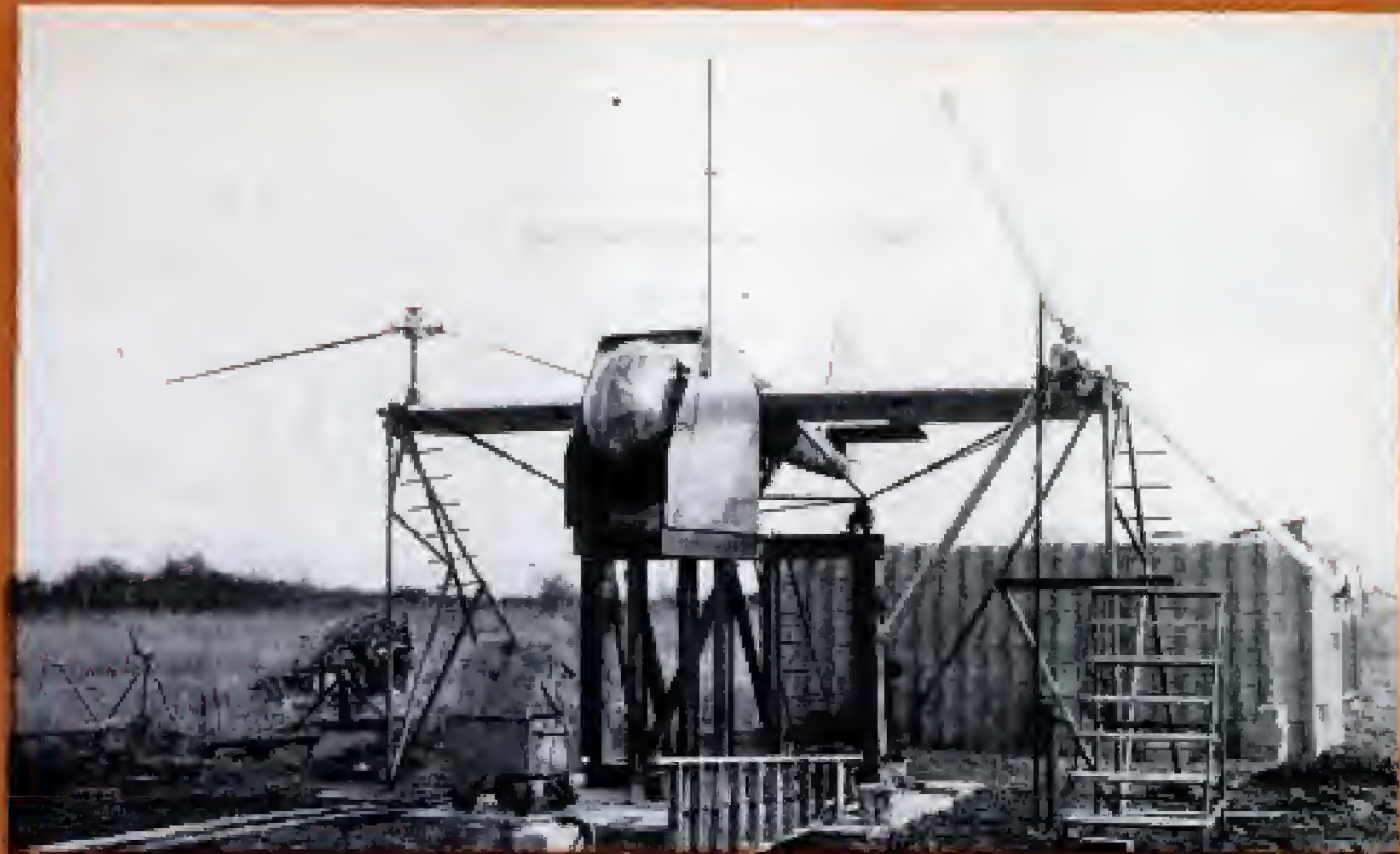
Transcendental's tiltrotor plane is still undergoing ground tests, will probably take to the air this year
